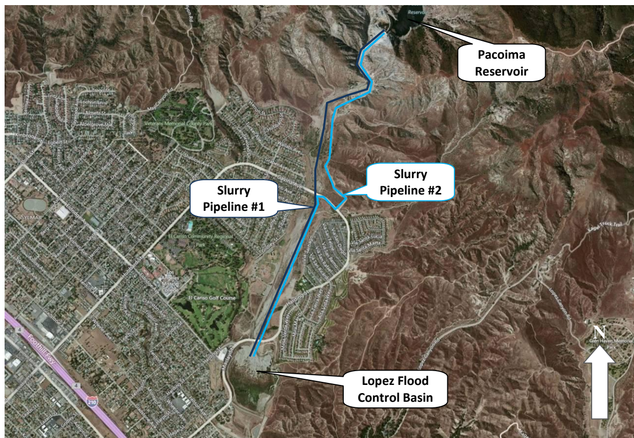
Figure 8-42 Potential Slurry Pipeline Alignments for Pacoima Reservoir
