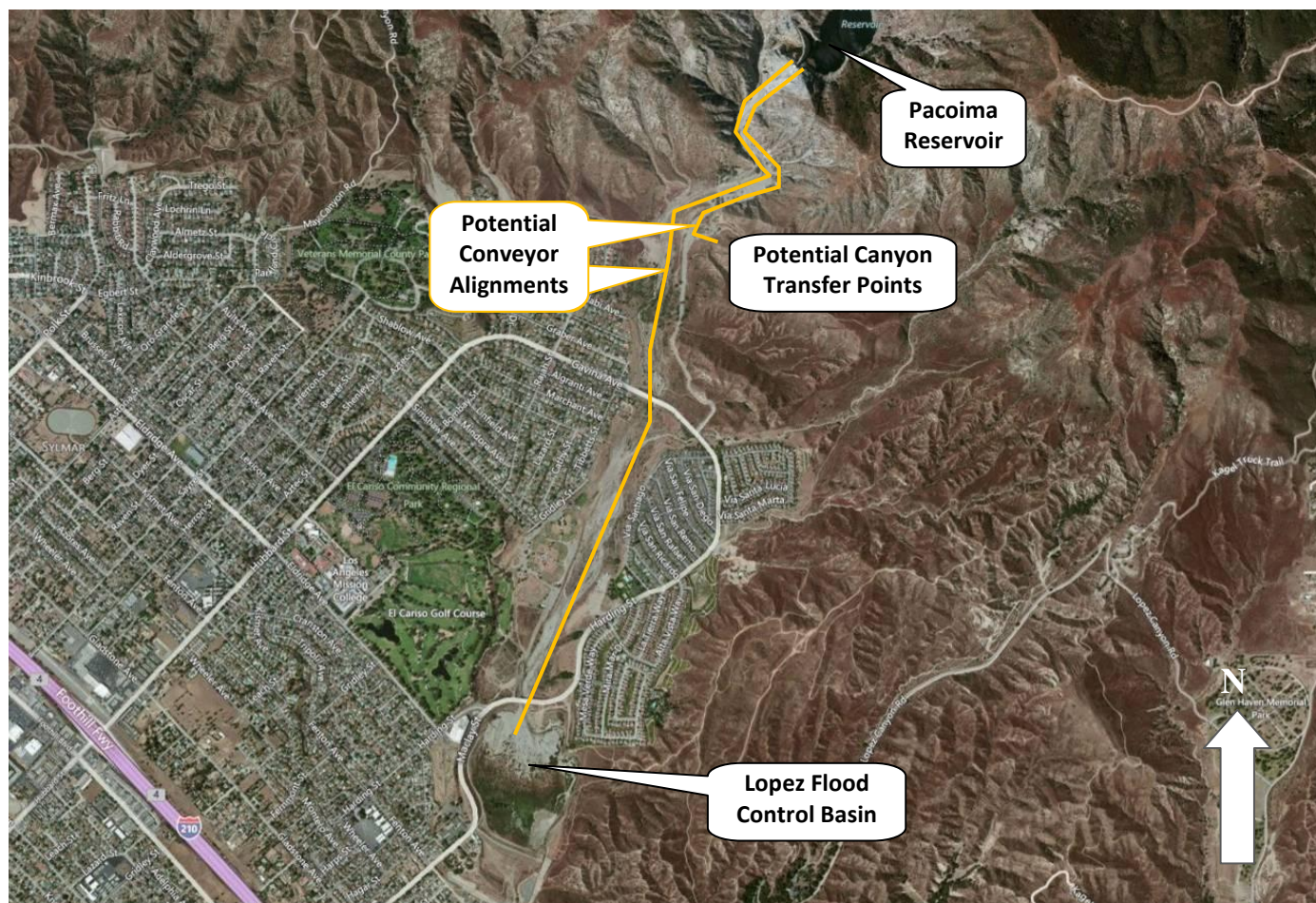
Figure 8-41 Potential conveyor belt alignments
